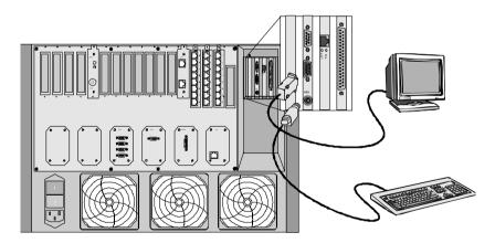
Figure 3-3: Attaching the Monitor and Key Board to the MGC-100
